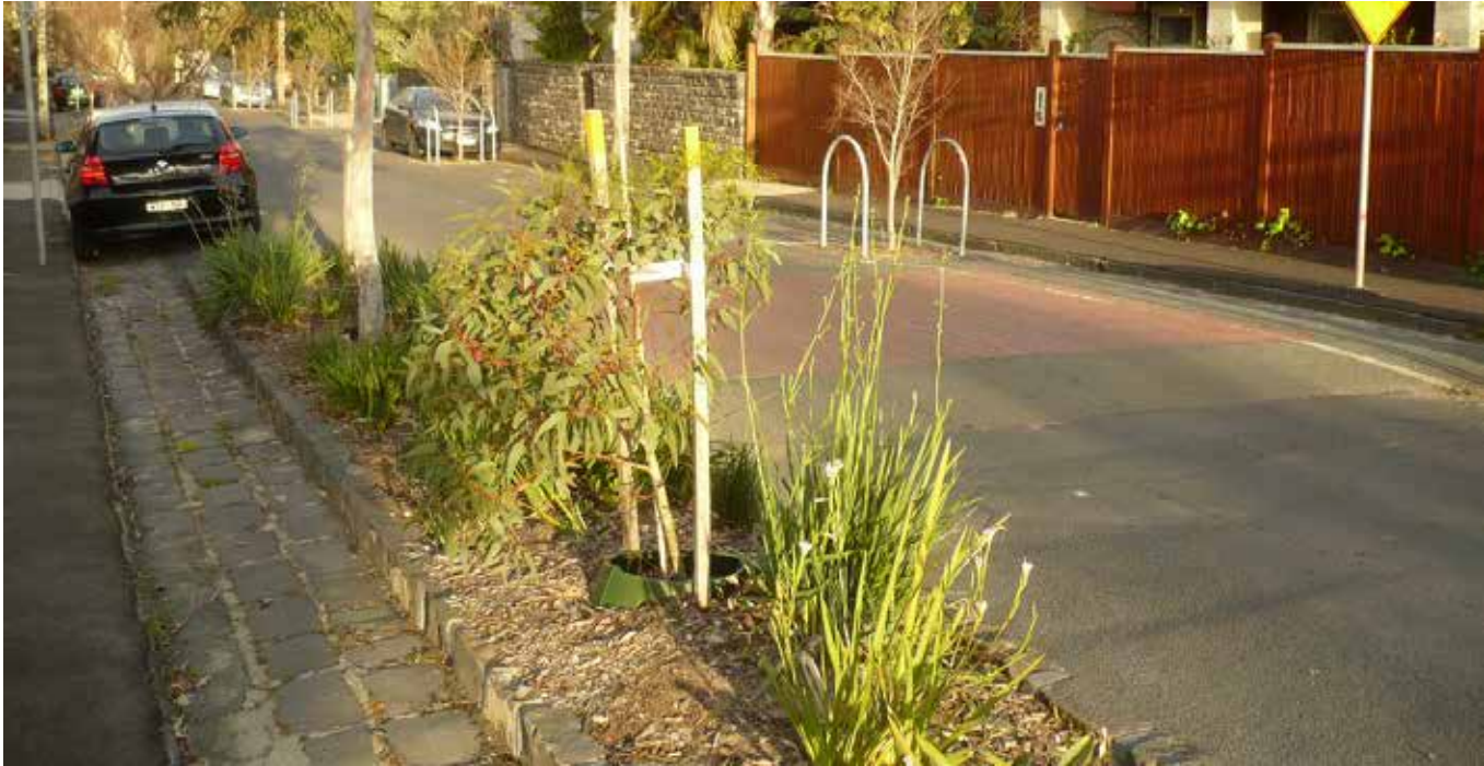
An example of a tree outstand in Octavia Street, St Kilda that is wide enough to plant two trees, providing benefits of connected soil and canopy (Image Credit Jaag St Kilda)
